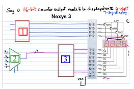
Now, if we want to display the output of a 32-bit binary counter as an 8-digit hexadecimal number going from 0000 0000 to FFFF FFFF on the 8 SSDs of a Nexys-4 board, what three components you intend to use?
