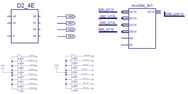
You can use a 2x4 decoder such as the above  $D2_4E$ . Look up the Xilinx library UG616 for the D2\_4E decoder to check if the enable input is active high or low and the outputs are active high or active low. We also provided you with the 8-bit wide 4x1 mux shown above. The diagrams on pages 18/29 to 20/29 (section 9.1 on Seven Segment Display) of the Nexys 4 reference manual will help you in understanding the scanning operation. Celebrate the completion of your lab!
