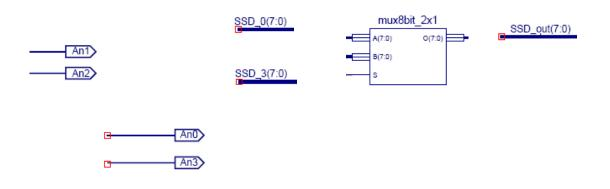
Method #2: Instead of permanently disabling AN1 and AN2 (as in Method#1), let us send Ca-Cg, Dp=11111111 to the 8 cathodes (remember these are active low so this will blank the displays). Now we need to activate the 4 anodes, one at a time in sequence, while sending the corresponding 8-segment information to the cathodes with a 8-bit wide 4-to-1 mux. You can use perhaps DIVCLK(15:14) for this purpose.
