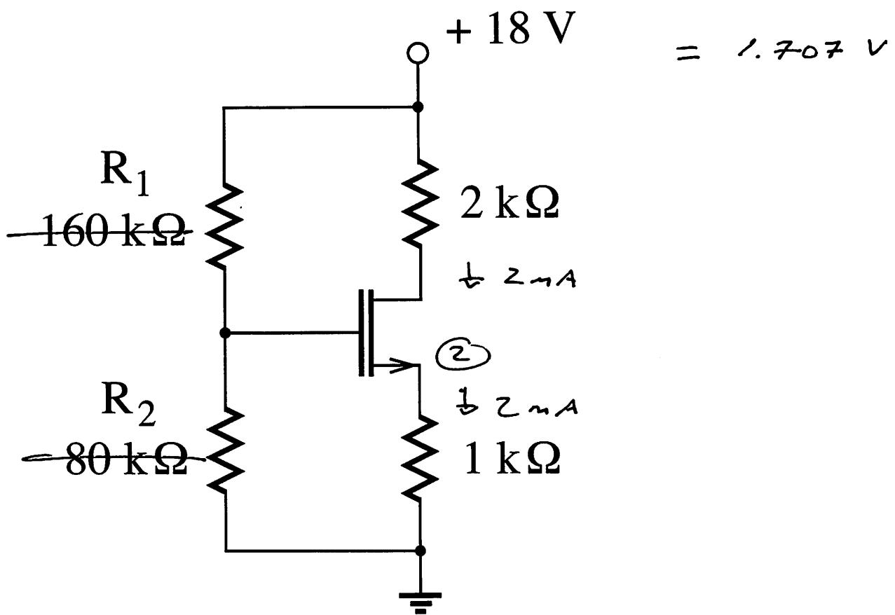
$$18 \left( \frac{r_2}{r_1 + r_2} \right) = 3.707 \quad \left. \begin{array}{l} \rightarrow r_1 = 100k \left( \frac{18}{3.707} \right) \\ r_1 = 486k \end{array} \right\}$$
