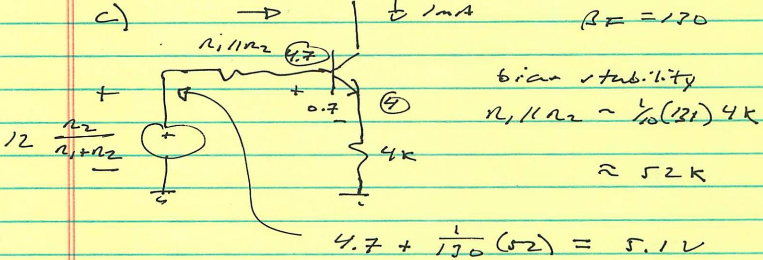
$$12 \frac{R_2}{R_1+R_2} = 5.1 \quad \left. \begin{array}{l} \\ \end{array} \right\} \rightarrow R_1 = 52\text{k} \left( \frac{12}{5.1} \right)$$
