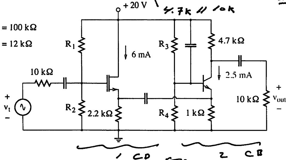
$$r_{in}^{(2)} = 1 \text{ k}\Omega \parallel \frac{r_{o1}}{1 + R_o} = 10.2 \text{ }\Omega$$
