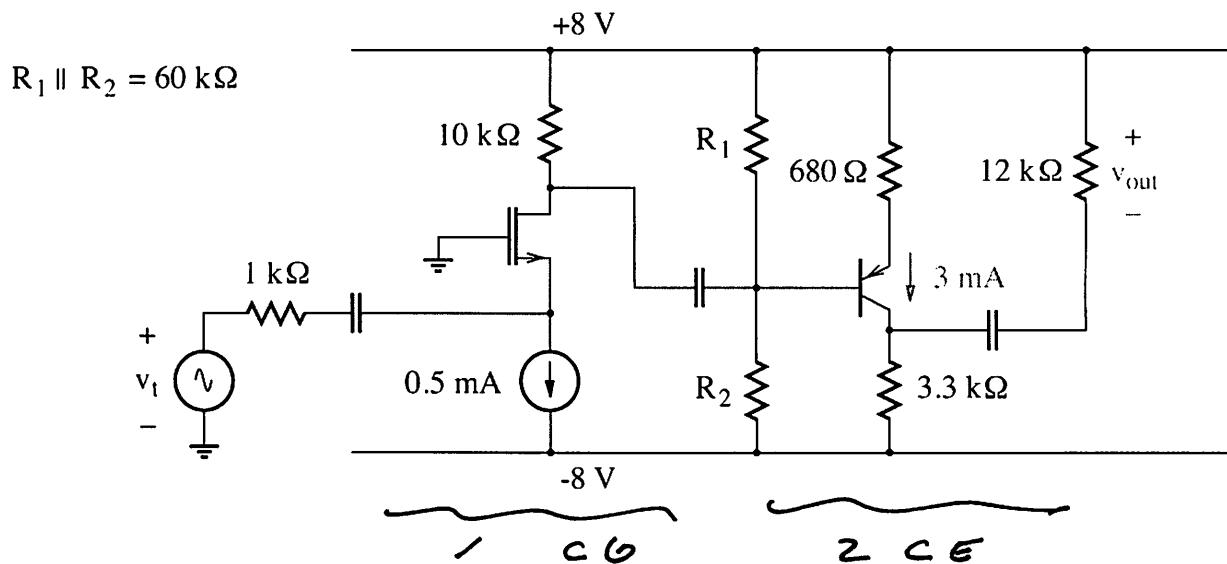
$$r_{\pi 2}' = 2.3 \text{ k}\Omega \parallel 12 \text{ k}\Omega = 2.59 \text{ k}\Omega$$
