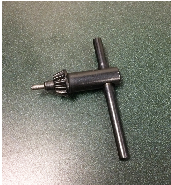
Figure 2: Chuck key for tightening the chuck around bits
