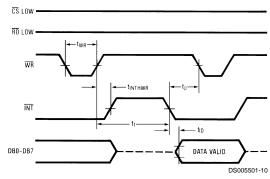
FIGURE 5. WR-RD Mode (Pin 7 is High) Stand-Alone Operation
