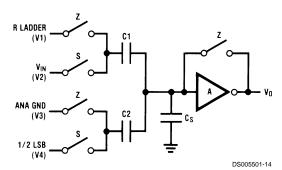
then made by connecting the second input on each capacitor and opening all of the other switches (S switches). The change in voltage at the inverter's input, as a result of the change in charge on each input capacitor, will now depend on both input signal differences.
