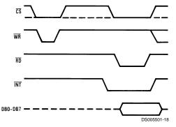
FIGURE 10. WR-RD Mode (Pin 7 is High and t<sub>RD</sub>>t<sub>I</sub>)
