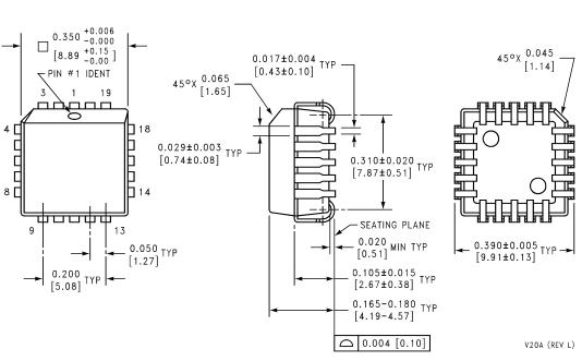
Molded Chip Carrier Package (V) Order Number ADC0820BCV NS Package Number V20A
