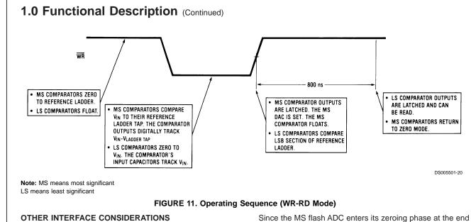
In order to maintain conversion accuracy,  $\overline{\text{WR}}$  has a maximum width spec of 50 µs. When the MS flash ADC's sampled-data comparators (Section 1.2) are in comparison mode ( $\overline{\text{WR}}$  is low), the input capacitors (C, *Figure 8*) must hold their charge. Switch leakage and inverter bias current can cause errors if the comparator is left in this phase for too long.
