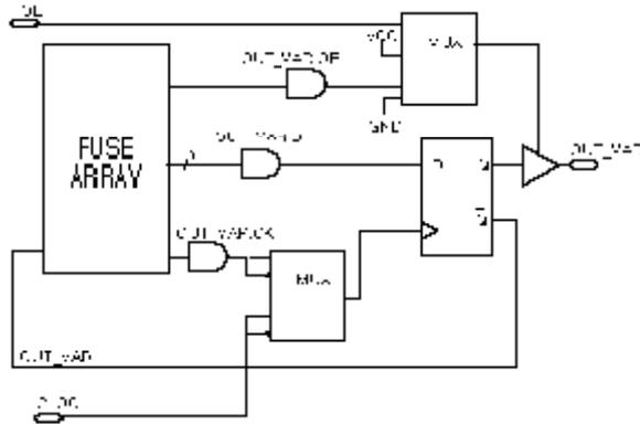
Figure 1.11: Output with Output Enable and Clock Multiplexers
