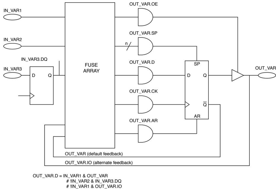
Figure 1.6: Circuit Illustrating Extensions
