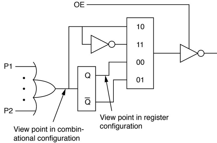
Figure 2.4: Observation Points Using Trace Level 4
