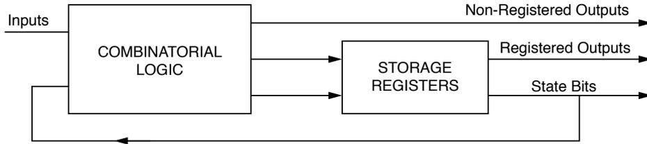
Figure 1.18: State Machine Model
