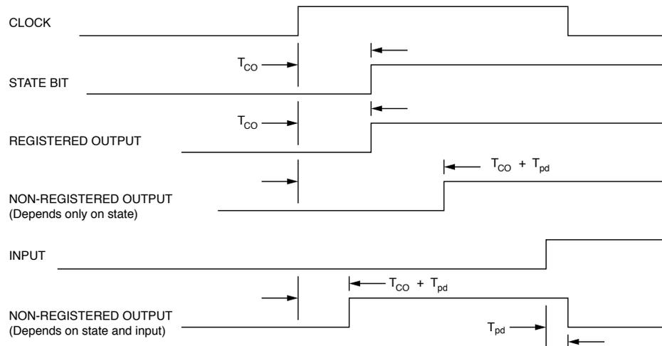
Figure 1.19: State Machine Timing Diagram
