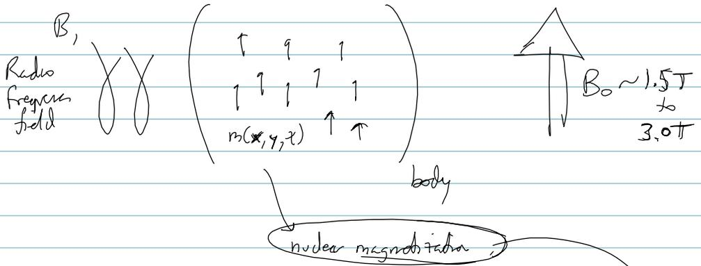
$B_0$ : polarizes the sample, creates a resonance condition
