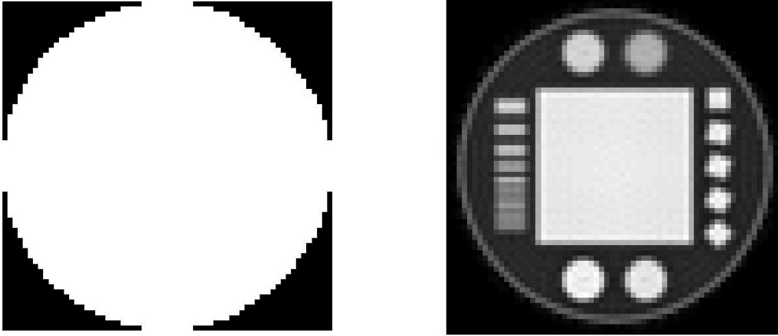
Figure 8: Morphological operations of erode, dilate and fill are applied to get the object mask representing the object support. After deleting the columns corresponding to blank pixels from the system matrix H , the image is reconstructed again iteratively for 5 iterations. We can see that the high frequency artifact is less severe (central square). Also the two disks on the top are better reconstructed resulting in better reconstruction compared to gridding.
